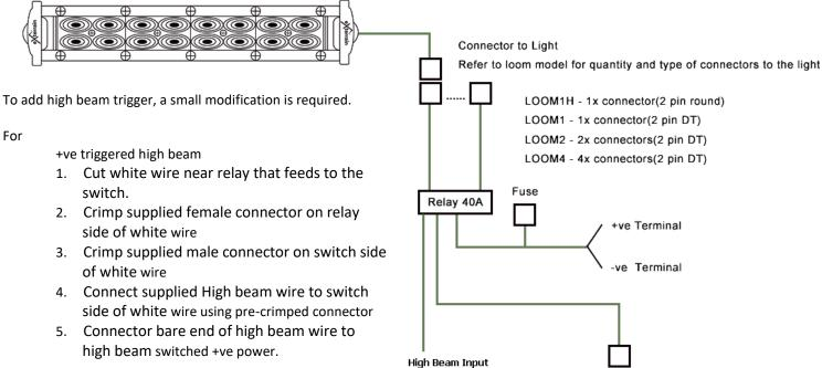
Please note: Drawing is an example only – wiring loom is not included with purchase of RAVEN bar lights. eXterrain wiring looms are available for purchase (see inset picture). All loom must be operated on 12 Volt only— LOOM1H (MAX 480W), LOOM1 (MAX 180W), LOOM2 (MAX 360W) AND LOOM4 (MAX 480W).
